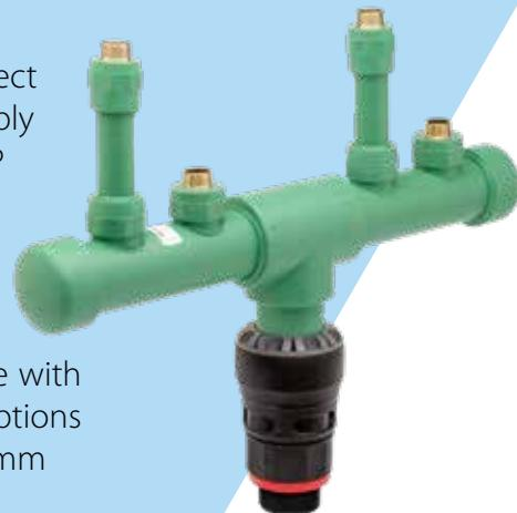
An extensive range of one piece construction manifolds are available with between 2 and 16 outlets, 2 different incoming supply connection options and a choice of a straight 130mm outlet arrangement, or a 90mm staggered option, both allowing installation of meters in accordance with the requirements of the water utility companies.
